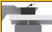
Arrow: Fasten through ridge cap & Uni-Vent® Pro-Series into purlin.
