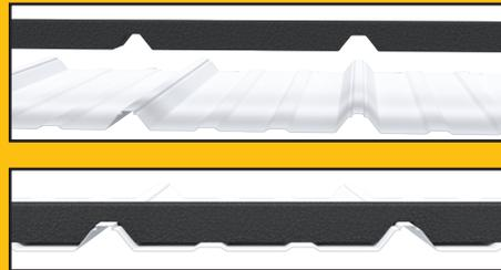
Roll out Uni-Vent® Pro-Series while aligning the ribs. After the Uni-Vent® Pro-Series is rolled out over the high ribs, the installer must press down between the high ribs for full adhesion.
